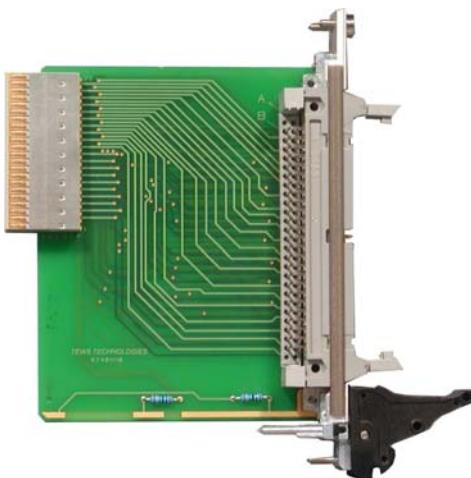
It distributes all 100 IP I/O lines from the cPCI RJ2 connector to two 50 pin ribbon cable connectors (stacked version) located in the front panel.
