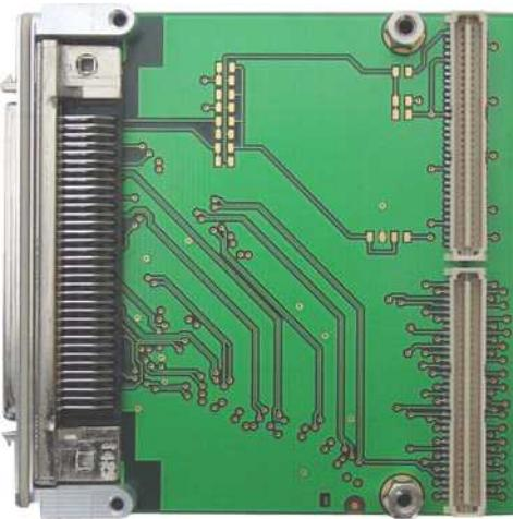
The TPIM005 distributes all 64 PMC back I/O lines to a 68 pin SCSI-3 type connector located in the EMI front panel. The routing and I/O signal mapping of the TPIM005 is optimized for differential pair routing.
