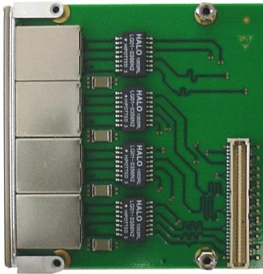
The TPIM006 distributes the Ethernet signals of the TEWS' Gigabit Ethernet modules with back I/O to RJ-45 connectors located in the front panel of the PIM module.
