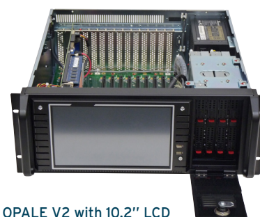
OPALE V2 with 10.2" LCD for telemetry control
