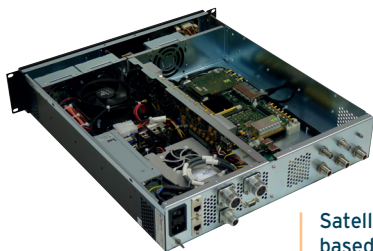
μOPALE V2-D NAS server with RJ-Field connectors
