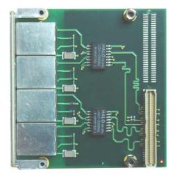
The TPIM004 provides access to the Fast Ethernet Ports of TEWS' Fast Ethernet PMCs with Back I/O like the TPMC882-1x or the TPMC382. Refer to the TPMC Data Sheets to find out, if the TPIM004 can be used with the corresponding PMC.
