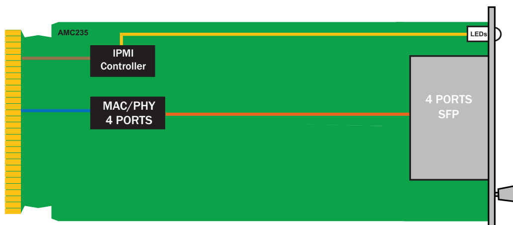
FIGURE 1. AMC235 Functional Block Diagram
