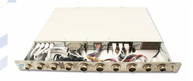
Front View of the VT858 with the cover removed
