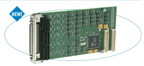
With eight serial ports per module, the PMC521 provides a high-density solution to reduce costs and use fewer card slots.
