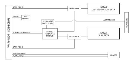
Boot via PCIe or SATA/SAS ◆ Supports dual SSD or a single 2.5" drive ◆ Dual SSDs are RAID 0/1 configurable
