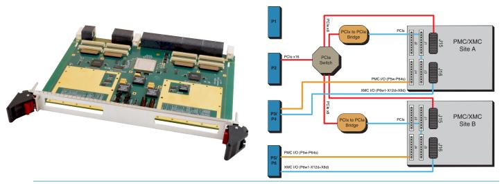
PCIe x8 Gen 2 interface via Expansion plane
