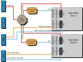
PCIe x8 Gen 2 interface via Data plane
