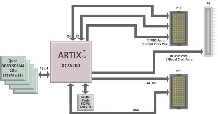
XMC module with PCIe interface ◆ Logic-optimized Artix-7 FPGA ◆ Conduction-Cooled
