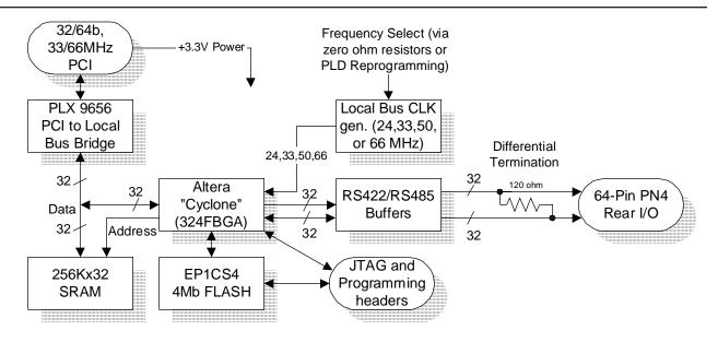
The Conduction Cooled 32-channel Reconfigurable RS422/RS485 Digital I/O PMC provides a vehicle for implementing complex user-specific digital designs requiring a differential interface. Thirty-two (32) general-purpose RS422/RS485 driven digital I/O differential pairs are wired to the rear PN4 connector. For each of the 32 channels, the bidirectionality is controlled by an output from the FPGA.
