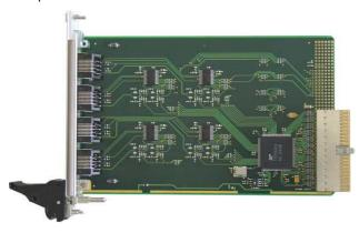
All modules offer front panel I/O with four RJ45 connectors. The TCP463-2x modules offer additional J2 rear I/O. Each RS232 channel supports TxD, RxD, CTS, RTS, DTR, CD, DSR/RI and GND. Each RS422 channel supports RxD+/-, TxD+/- and GND on front and RxD+/-, TxD+/-, RTS+/-, CTS+/- and GND on rear I/O.
