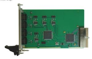
The serial channels can be individually programmed to operate as RS232, RS422 or RS485 full duplex/half duplex interface. In addition programmable termination is provided for the RS422/RS485 interfaces. After power-up all serial I/O lines are in a high impedance state.
