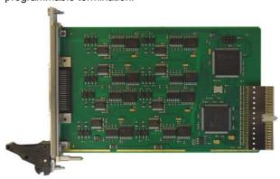
Each RS232 channel supports RxD, TxD, RTS, CTS and GND. RS422 and RS485 Full Duplex support a four wire interface (RX+, RX-, TX+, TX-) plus ground (GND). Half Duplex supports a two wire interface (DX+, DX-) plus ground (GND).
