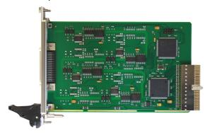
Each serial channel can be programmed via a CPLD register to operate as an RS232, RS422 or RS485 interface. The RS422 and RS485 interfaces can be programmed as Full Duplex or Half Duplex interface with programmable termination.
