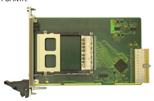
The power management unit provides 3.3V or 5.0V PC Card power supply and 3.3V, 5.0V or 12V PC Card programming voltage. Due to the short circuit and thermal protection of the power management unit no external fuses are needed on the module.
