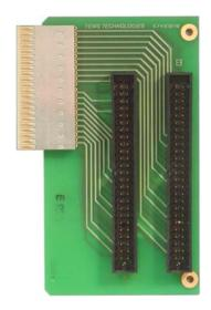
It distributes all 100 IP I/O lines from the cPCI RJ2 connector to two 50 pin ribbon cable connectors allowing easy rack internal wiring.
