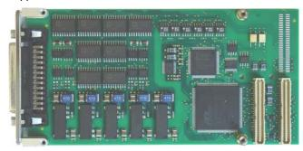
A sequencer allows periodical updates of enabled channels and the sequence timer range extends from 100µs to 6.5s.
