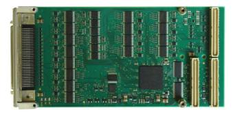
To eliminate spikes and glitches, keeping interrupts to a minimum, each port has its own user configurable input filter.
