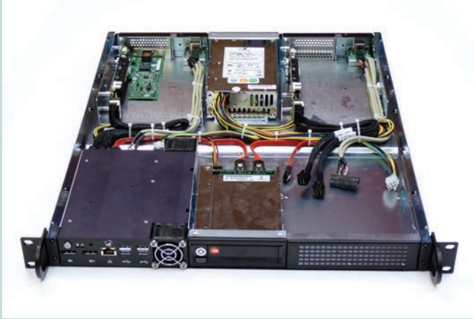
Figure 4: Two redundant myOPALE building blocks in a 1U/19-inch rack mount
