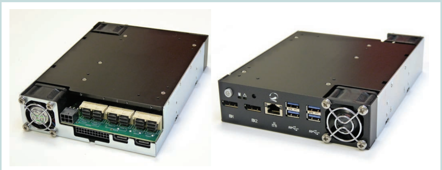
Figure 1: The myOPALE-CPU building block with its six Mini-SAS HD connectors and 24 PCIe Gen3 links
